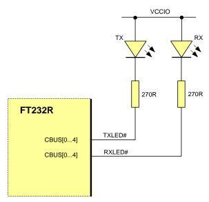
Figure 7.5 Dual LED Configuration
