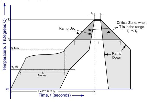
Figure 9.5 FT232R Solder Reflow Profile
