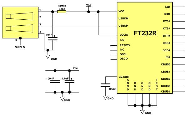
Figure 6.1 Bus Powered Configuration
