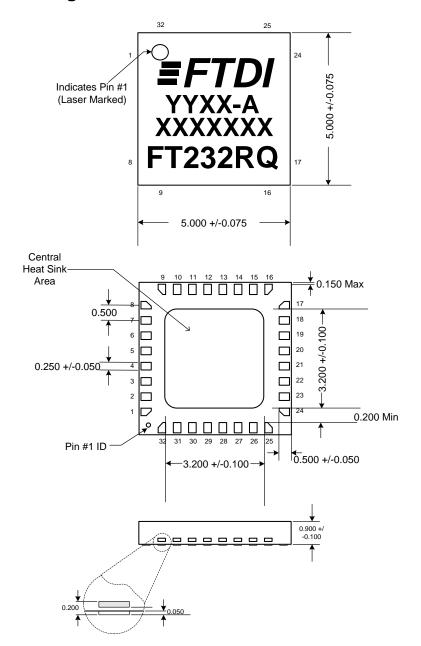
Note: The pin #1 ID is connected internally to the device's central heat sink area. It is recommended to ground the central heat sink area of the device.
