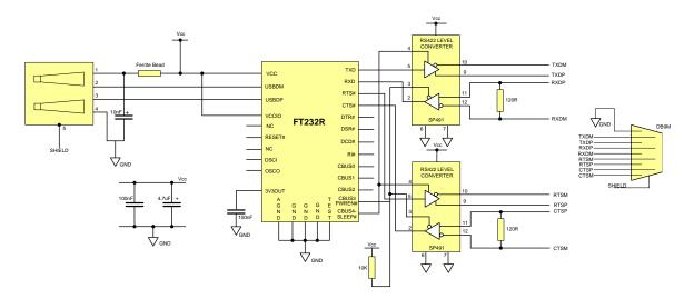
Figure 7.3 USB to RS422 Converter Configuration
