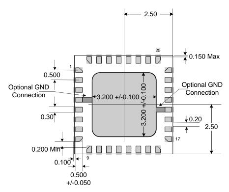
Figure 9.3 Typical Pad Layout for QFN-32 Package
