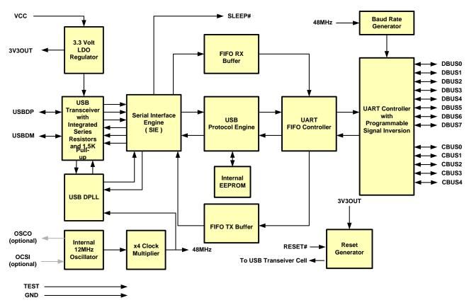
Figure 2.1 FT232R Block Diagram
