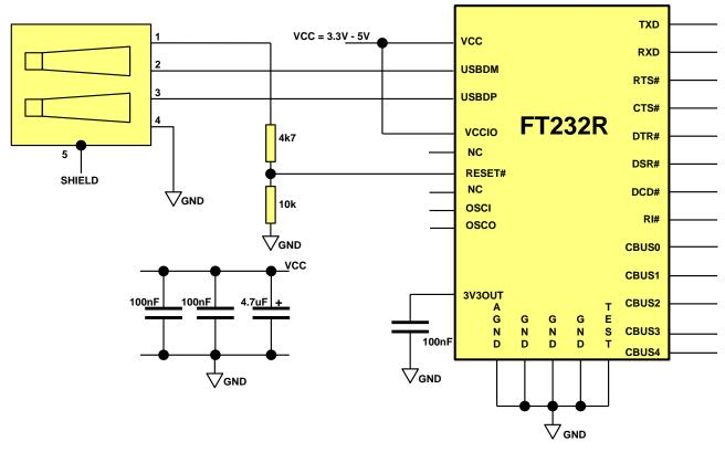
Figure 6.2 Self Powered Configuration
