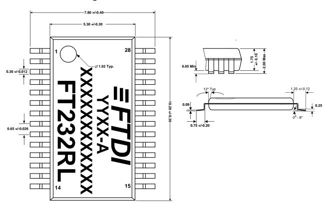
Figure 9.1 SSOP-28 Package Dimensions
