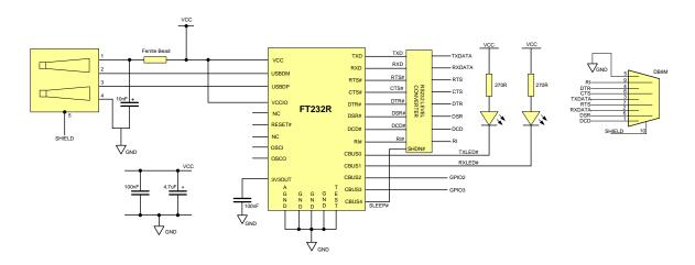
Figure 7.1 Application Example showing USB to RS232 Converter
