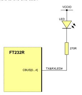
Figure 7.6 Single LED Configuration
